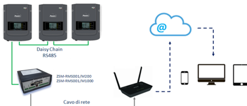
Figure 78 – Diagram showing the operation of the ZSM-RMS001/M200 / ZSM-RMS001/M1000 datalogger
