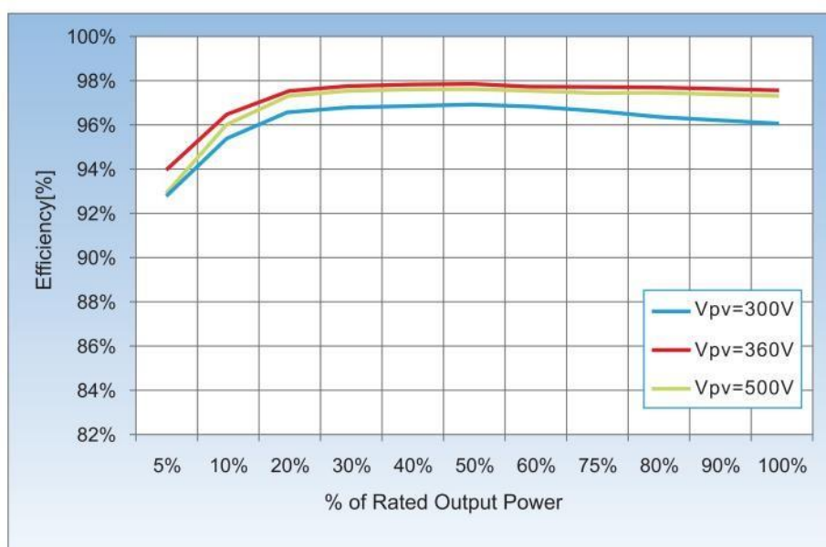
Figure 7 - Power efficiency curve
