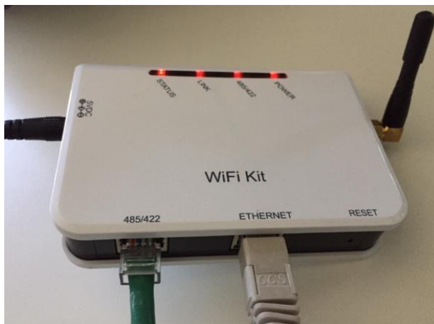
Figure 85 – Ethernet cable connected to the datalogger
