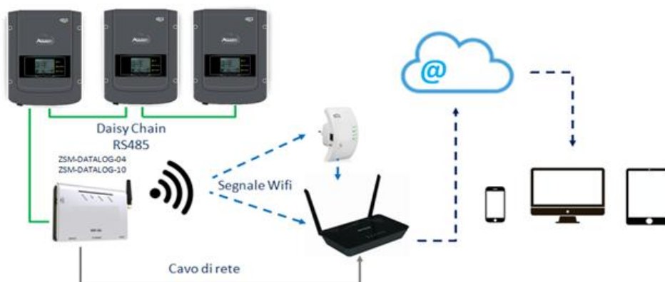
Figure 73 – Diagram for connecting the ZSM-DATALOG-04 / ZSM-DATALOG-10 datalogger
