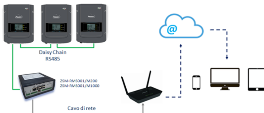
Figure 74 – Diagram showing the operation of the ZSM-RMS001/M200 / ZSM-RMS001/M1000 datalogger
